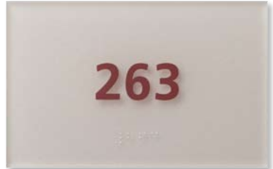
Clear acrylic, with maroon raised text, grade-2 domed Braille, stipple surface and beige second-surface
