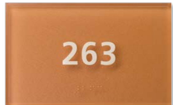
Clear acrylic, with raised text, grade-2 domed Braille, stipple surface texture, painted second-surface and polished, beveled edges.
